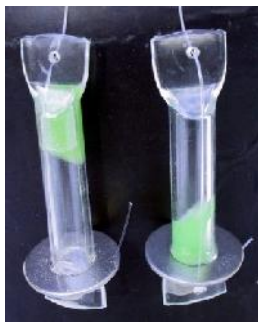
Fig. 1 Water Pasteurization Indicator (WAPI). Before heating water, wax at the top of the tube (Left). After water being pasteurized, wax at the bottom of the tube (Right) [8]
