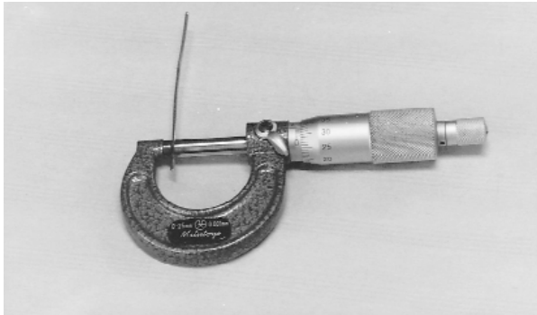
Fig. 3.23 Measuring diameter of wire
