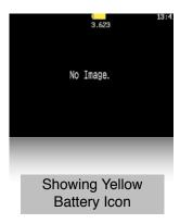
Set the maximum and minimum voltages to match fully charged and discharged batteries, the battery icon fill color will reduce as voltage lowers and will change to red color close to minimum voltage.
