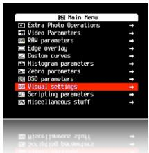
Like Canon's menus, pressing the FUNC.SET button will select the highlighted menu option. Pressing the DISP. button will move back one menu level. Pressing the MENU button will exit the current operation.
