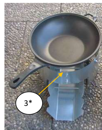
Fig. 1.6. Ben 3 with stove shell (3*) with 150 mm height for pan/wok
