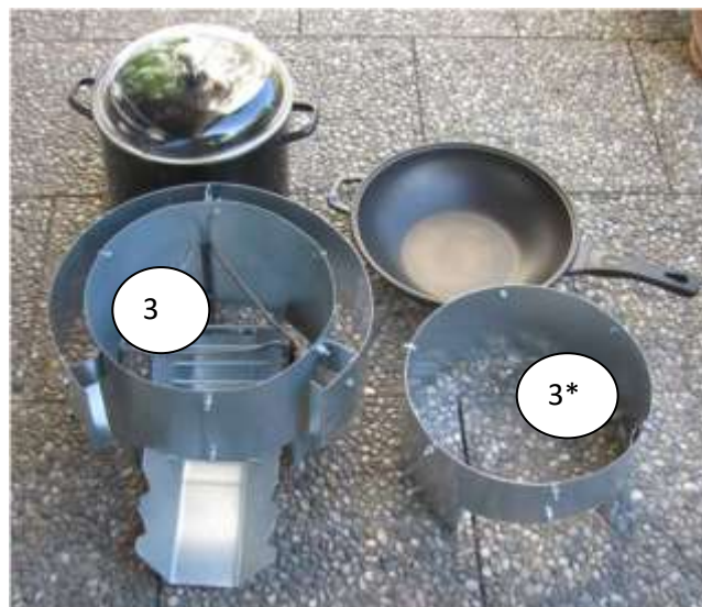
Fig. 1.5. Ben 3 with stove shell (3) with 200 mm height for pot and (3*) with 150 mm height for pan or wok
