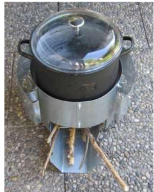
Fig. 1.2. Ben 2 with 28cm pot. Fuelwood sticks may be hold at cuts on the top edge of the ash pan.
