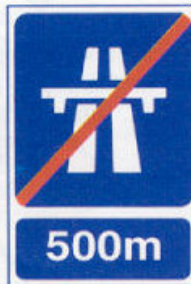
Approaching end of motorway
